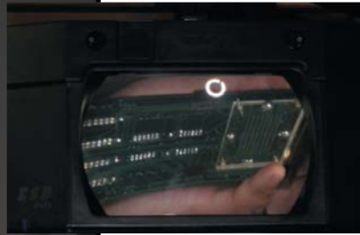
Close-up of Yen's transducer, the largest ever built, with over 65,500 individual elements, 169 transmitter elements and 1,024 receiver elements. That gives it four times the imaging sensitivity of previous arrays.
