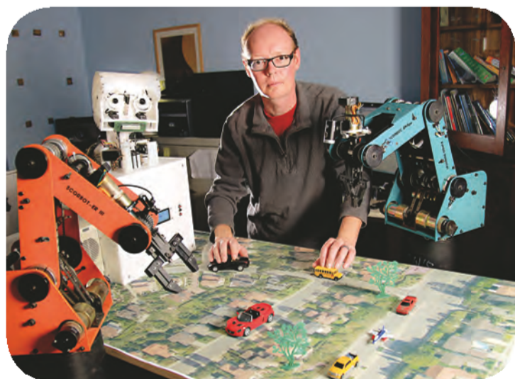
Laurent Itti with a robotic-assisted scenery model used to train and test neuroscience-inspired machine vision algorithms. One robot arm controls the position of the sun, while the other moves objects around the scene. This creates hundreds of thousands of new scenarios for observation and analysis by the vision algorithms.
